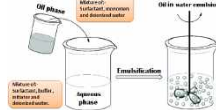
Schematic Representation of Emulsion Polymerization Process
