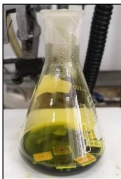
Figure 3. Acid leaching of waste SIM cards
