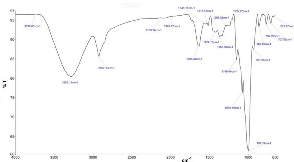
**Figure 3** FTIR spectra of field grown plant-AgNPs (W-AgNPs)
