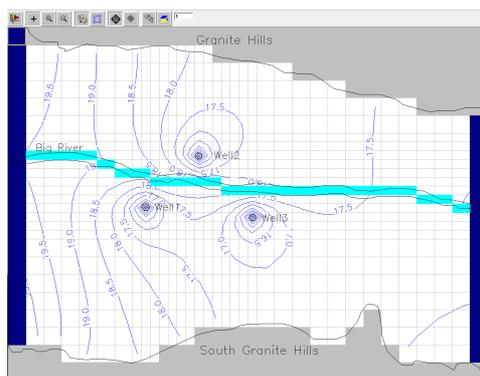
**Figure 3:** Steady-state head distribution in the first model layer
