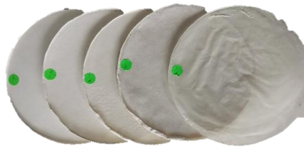
Fig. 6 NFC filter paper fabricated from Neolamarckia cadamba
