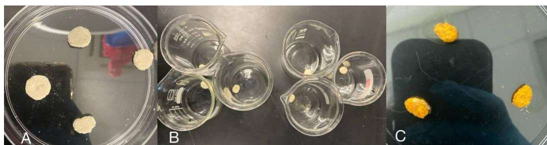
Figure 4 (A) 50 mg of CMC hydrogel (B) 50 mg CMC hydrogel in each beaker (C) Curcumin-loaded CMC hydrogel
