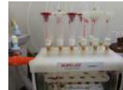
Solid Phase Extraction of Determination Organochlorine Pesticide
