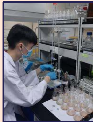
Chemical Oxygen Demand Test
